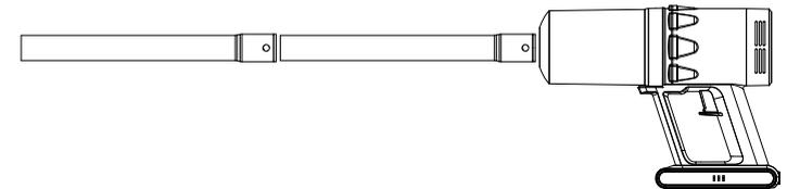
Connect the connecting pipe component with the ground brush as shown in the figure, insert the appropriate depth and fix it by friction. The ground brush can be installed in place and used. Used for cleaning floor and other objects
