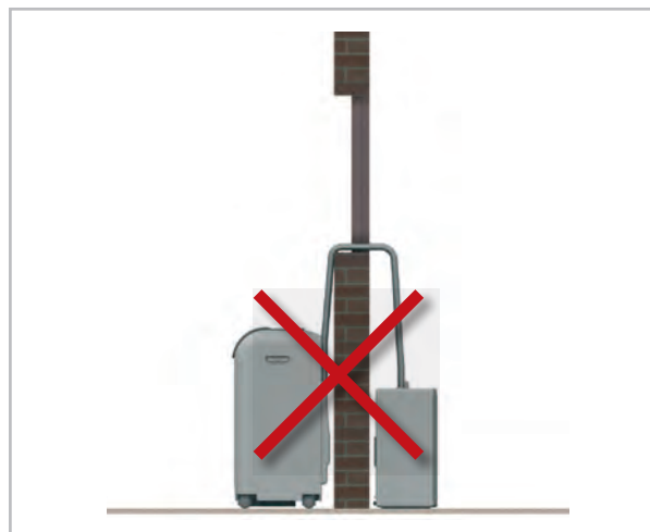
Fig. 6: Absence of minimum gap
