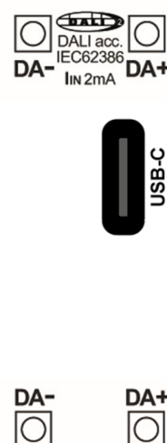
connection plan DALI-2 USB Pro 30mA HS
