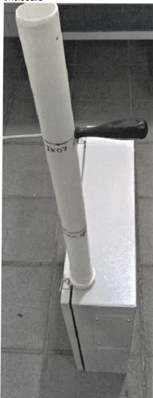
Picture 6. IK07 test set up for right side of the enclosure
