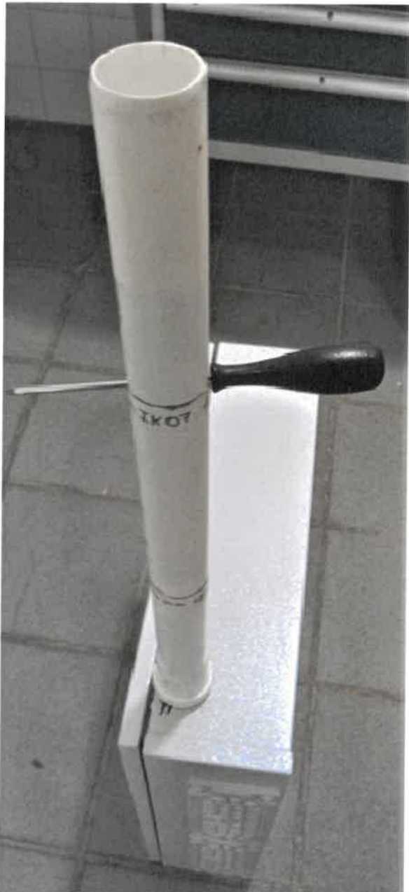
Picture 5. IK07 test set up for left side of the enclosure
