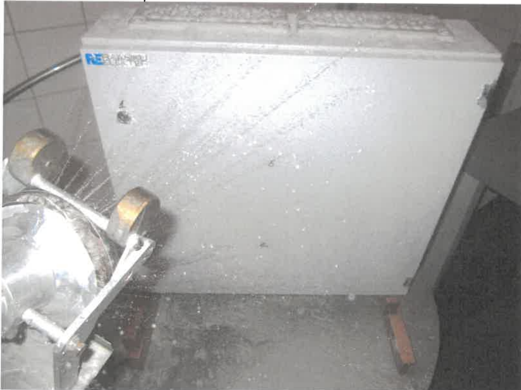
Picture 13. Test set up IPX4
