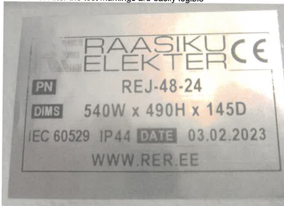
Picture 19. After the test markings are easily legible
